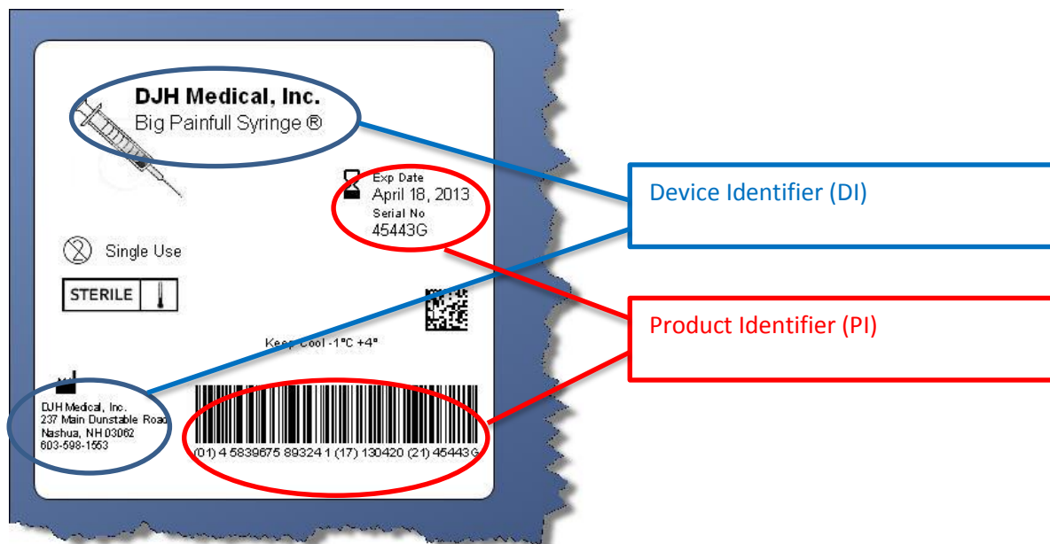
Fig 1: Illustration of an example of UDI compliant labelling incorporating VDP to facilitate individualization.
